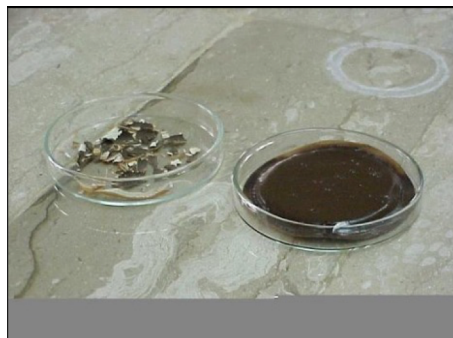
Result with OBM cake: Before (right) and after (left) HDC Mk II treatment for 6 hrs @ 90 °C gave 95% dissolution.
