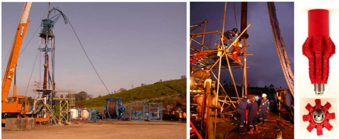
Figure 4: TFO Stimulation - Coiled Tubing (2-in OD coiled tubing) Operation
