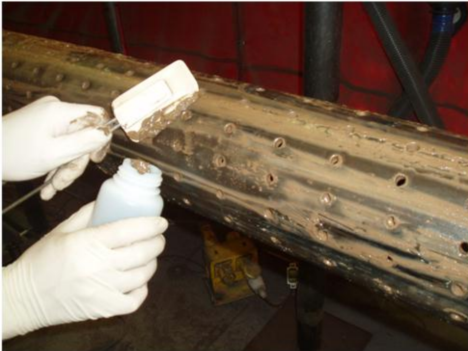
Picture 3: sample of mud solids being retrieved from the base pipe of the screen from the aborted 1 st completion run for lab analysis.
