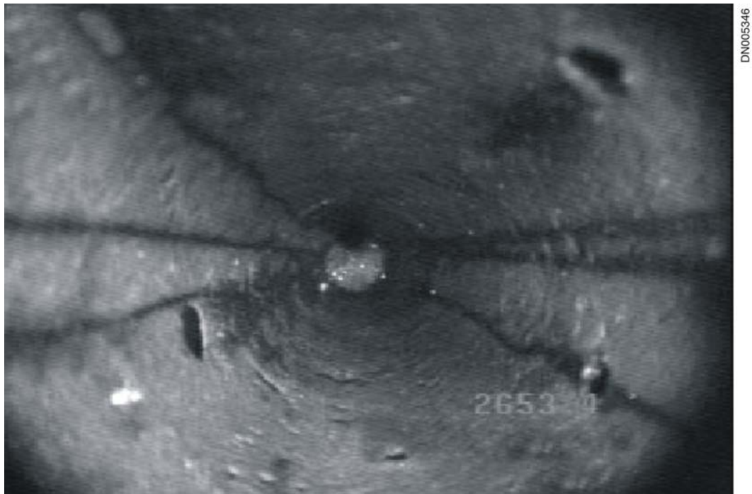
Fig. 8— Elk City 1 well video after CT cleanout.
