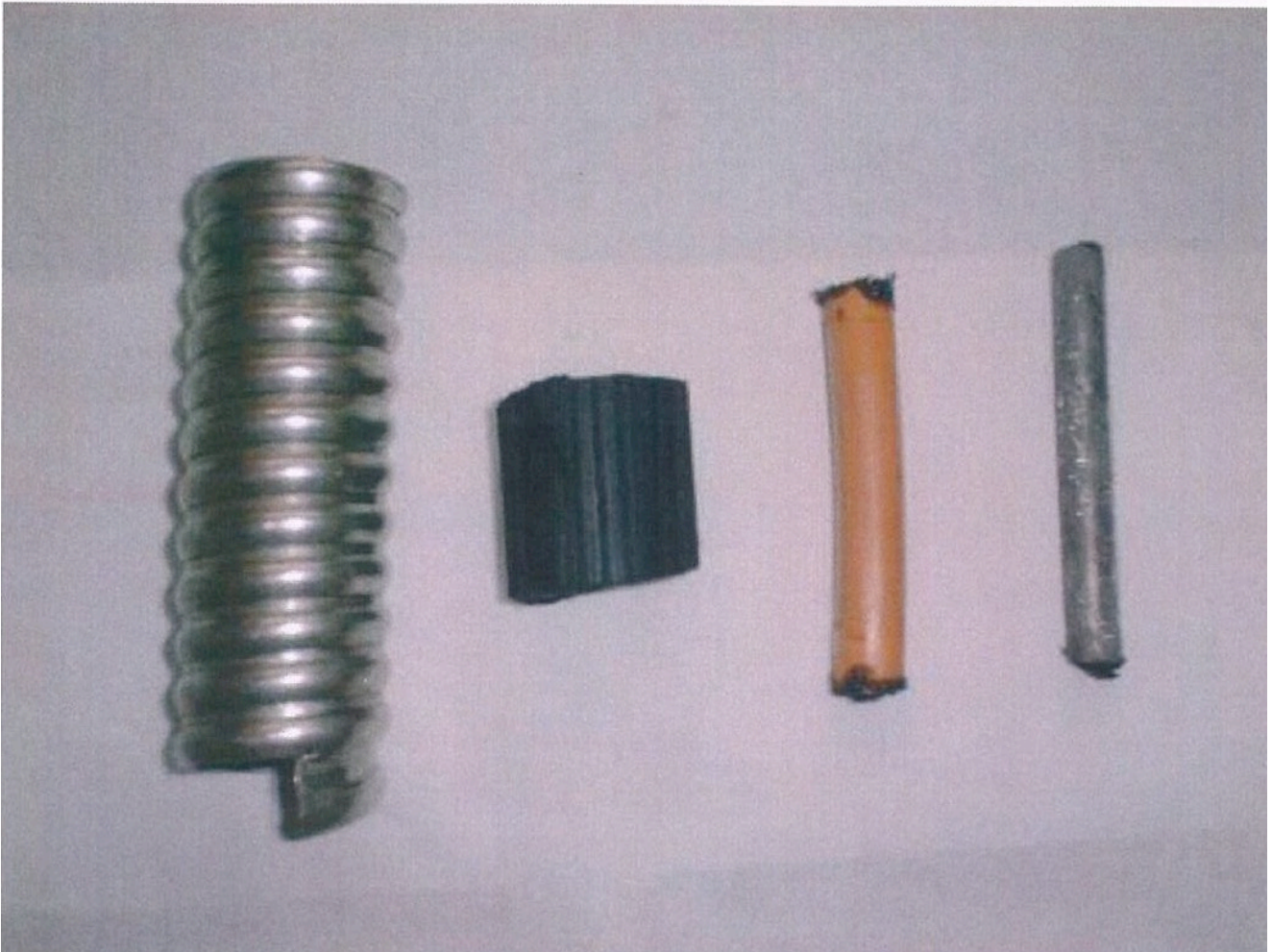
Photo 2: Post Static Aging - note pitting on lead wire surface; discoloration at wire ends due to absorption of product on epoxy resin sealant
